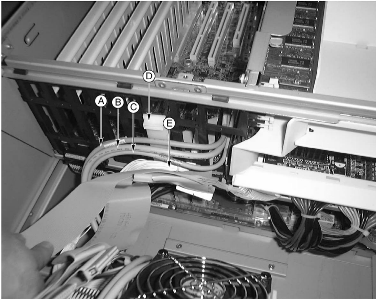
Figure 11 - Rear cables in the cable clamp
